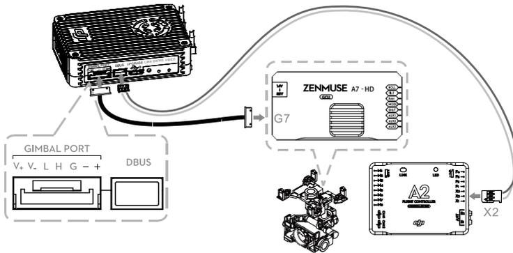
This example is based on a Z15-A7 gimbal and the A2 flight control system.
