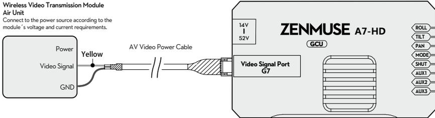
1. Solder the AV Video Signal and GND cables to the wireless video transmission module (Air Unit) as shown above.
