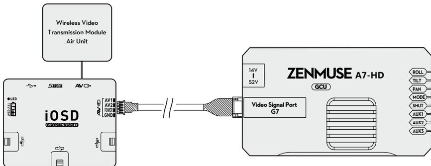
1. Connect the iOSD Mark II cable to the GCU's G7 port.
